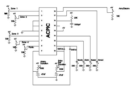
This example does not make use of the momentary Arm/Disarm feature. To do so, ground pin 18, free pin 3 and clock pin 3 to arm or disarm. This circuit only uses LEDs as controlled devices. The following depicts use of a PIEZO buzzer and relay
