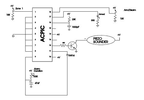
In all applications, the resistor and capacitor on pin 14 determine the part's clock frequency. This should approximate 32767Hz. A higher frequency will result in shorter debouncing times, entry exit and alarm delays. It will also cause the part to consume more power. Too high of frequency, and the part may not function at all. Too low of a frequency may result in the part not responding quickly enough to a sensor input and exit, entry and alarm delays which are too long.
